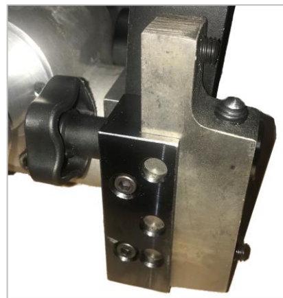
Properly Installed Rail Shoe
